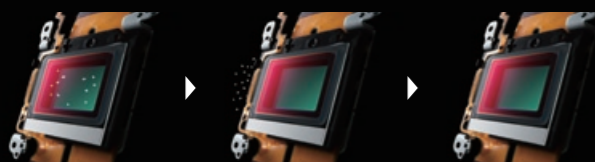
Flow of the Dust Reduction System
