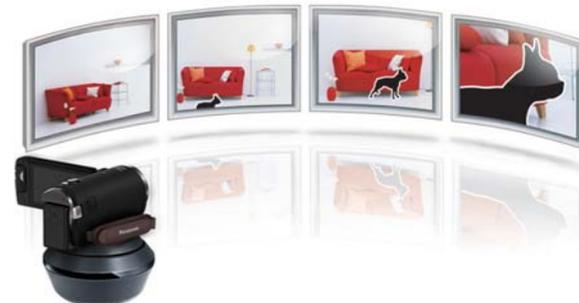
The motion sensor will find and follow your pet. If the pet stops moving for a while, the camera will zoom in. And if the pet is not found, the camera will search for it.
