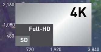
With four times the resolution of Full-HD, the WX970 and VX870 Series record in 4K [3,840 x 2,160] formats. This delivers true-to-life images for a wide variety of shooting situations, in extremely high detail.
