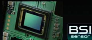
Increasing the readout speed has made it possible to handle large-volume 4K data. This suppresses the rolling shutter distortion that often occurs when shooting moving subjects.
